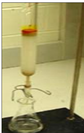
Fig 1: Transfer of adsorbent to column
